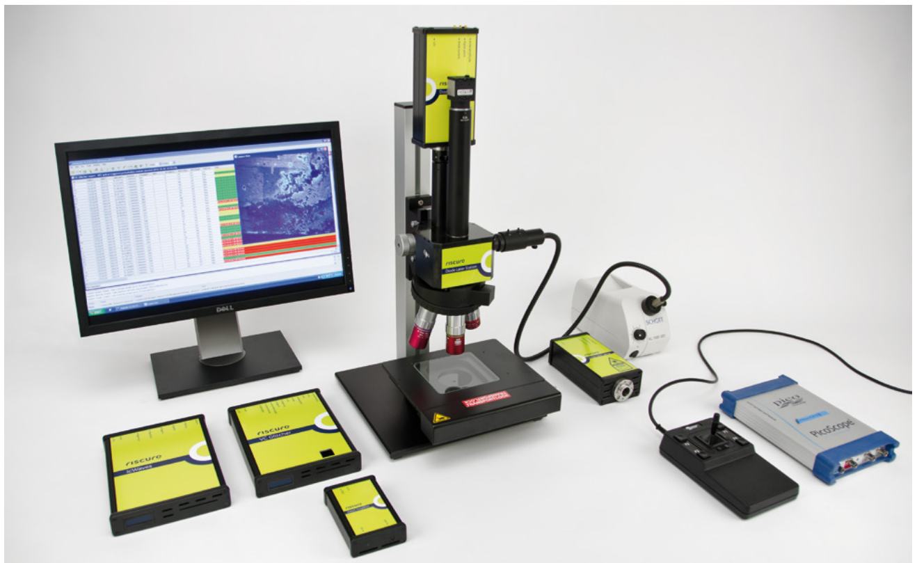
Inspector FI with VC Glitcher, icWaves, Glitch Amplifier and Diode Laser Station.
